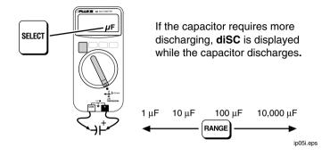
Note correct probe polarity for polarized capacitors.
